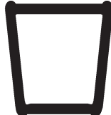
"Trapezoidal with teeth" crimping form
