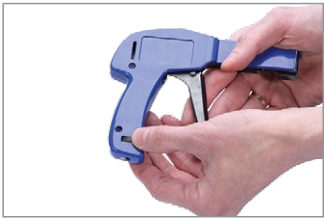
2.1 - Tightening the cable ties with a tool - set the max tension of the tool depending on the size of the tie
