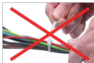
1.3 - Avoid sharp bending of the tie it will not improve the fixing strength
