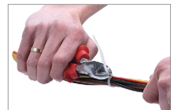
1.4 - Cut the exceeding part of the tie with the tool, leaving a few mm length as safety
