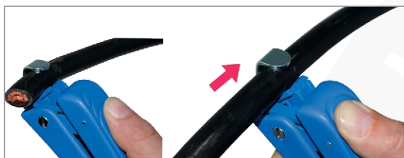
Stripping external insulation
