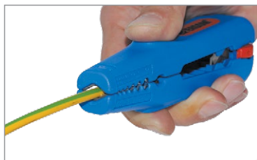
Circumferential stripping of wire external insulation
