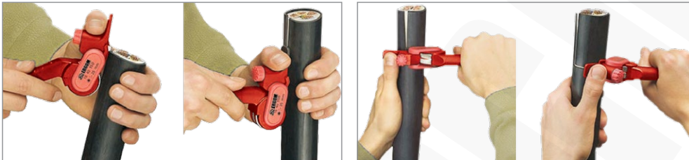
Longitudinal insulation cutting
