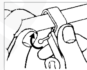
Change the direction of cutting by turning and holding the lever "A".
