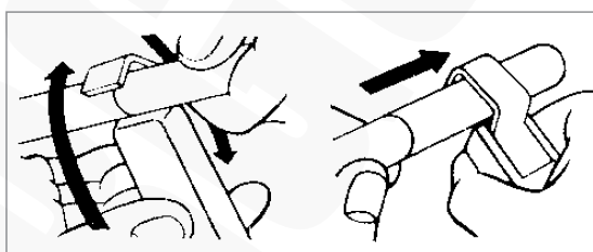
Stripping insulation from the end of cable
