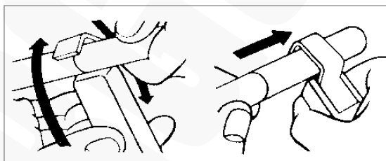
Stripping insulation from the end of cable
