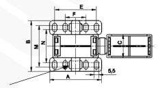
Gap on cable ties. (Max tie width 9 mm)
